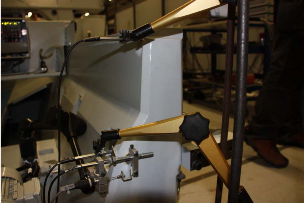
Fig. 1: Displacement measurements on the component cross-section under load
